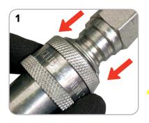
**1.** Attach the female quick connect fitting on the hose, to the male quick connect fitting on the product. Pull back the sleeve and apply slight force to mate the connectors.
