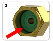
**2.** Place the plastic washer inside the fitting that connects to the tank, then attach the fitting. Tighten with the supplied tool, or any adjustable wrench (1 1/8").
