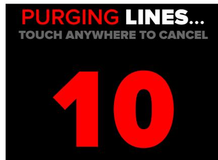
All valves will be opened for 10 seconds. User can disable purge at any time by touching anywhere on the LCD screen.
