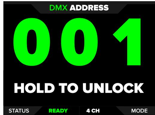
If screen is tapped when in idle state, user will be prompted to unlock fixture before settings can be changed.
