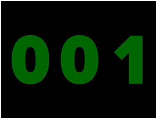
The display will dim when idle for 30 seconds with active DMX signal.
