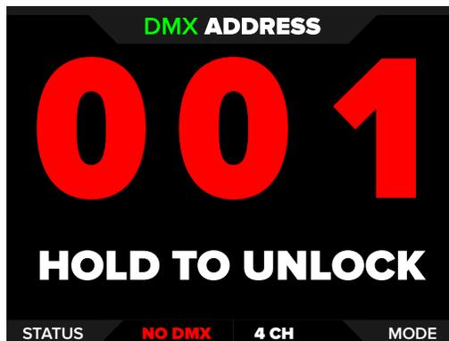
Alternatively, if there is no active DMX signal, idle state flashes display on unlock screen.
