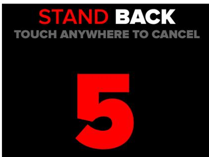
There will be a 5 second delay after activating the purge lines feature. This allows the user sufficient time to step away from the unit.
