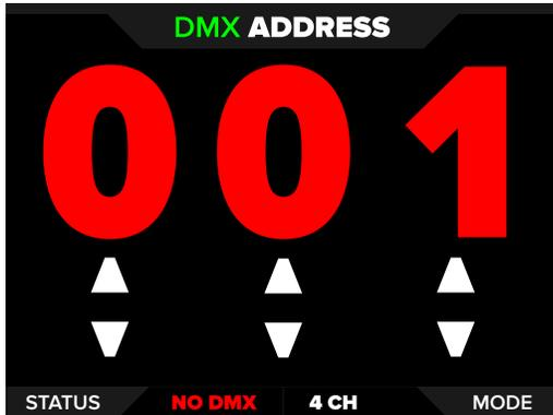
When no DMX is being received, the address will be displayed in red.
