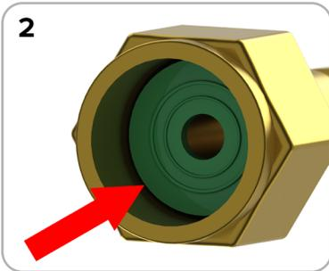
**2.** Place the plastic washer inside the fitting that connects to the tank, then attach the fitting. Tighten with the supplied tool, or any adjustable wrench (1 1/8”).
