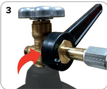
**3.** Position your CO<sub>2</sub> tank in a nearby location. Make sure the tank is stable, and won't tip over. Tanks should be secured with ratcheting straps or chain to ensure they are secure.
