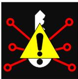
**E-Stop Triggered:** This icon shows a yellow caution icon, indicating that an emergency stop has been triggered, and all Key Triggers are currently disabled. This is a safety feature that allows users to quickly and easily shut down all SFX devices in case of an emergency. Tapping on the status icon will allow reactivation of the key triggers.
