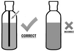
All Club Cannon® Products operate with a Siphon Co2 Tank. Using a standard Co2 tank will not produce the desired effect.
